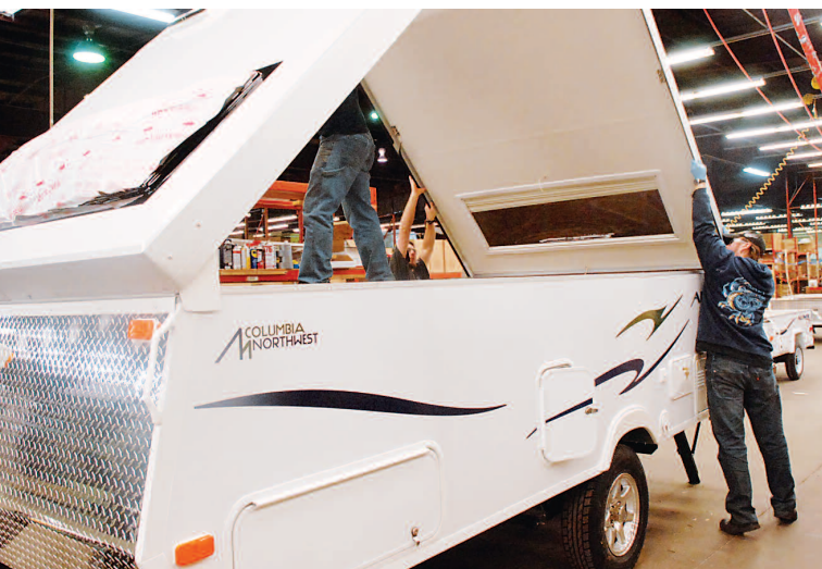
TOP: Worker Bill Riggs prepares an Aliner for A-wall installation. ABOVE: Ted Hall and Riggs separate roof panels to allow the A-wall to be fitted. RIGHT, TOP: As seen by this interior, while the lightweight Aliner is small enough to be towed by even a six-cylinder-powered family sedan, the units are well-equipped. RIGHT, BOTTOM: Ned Collins discusses production issues with Sean Smith, Columbia Northwest's line supervisor.
